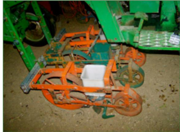
*Figure 24: This Planet Jr. seeder provides consistent spacing for crops that are sown directly into the ground.*
