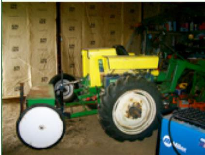
*(c) The Hefty G is used for planting (both seeding and transplanting) and for fertilizing. This tractor was converted to an electric motor in 2008. The Gandy fertilizer spreader is attached to the back of the tractor.*
