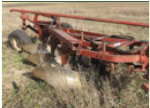
*Figure 40: Loon Organics' three-bottom (or moldboard) plow, used for initial cultivation of fields to prepare for sowing or planting.*
