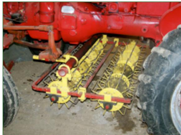
*Figure 25: This basket weeder maintains the same spacing as the seeder during cultivation for weeds.*
