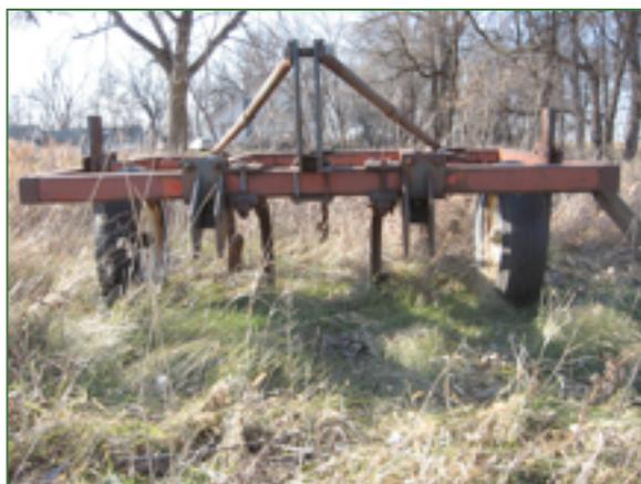
*Figure 39: A chisel plow accomplishes deep tillage without inverting the soil.*
