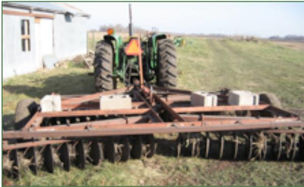
*Figure 37: A disc plow, or disc, uses one or more rows of concave discs to work the soil without turning it over completely.*
