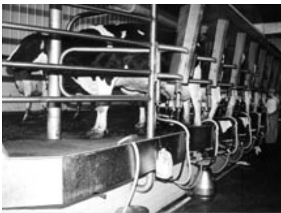
This fully-automated double-16 herringbone parlor can milk about 100 cows an hour.
