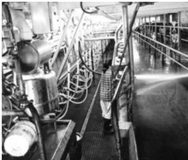
This operation modernized by adding a pit parlor, which improved labor efficiency and milker safety.
