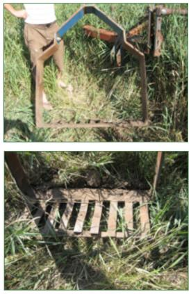
Figure 33: Loon Organics' root digger, shown in full view (top) and close up (bottom).
